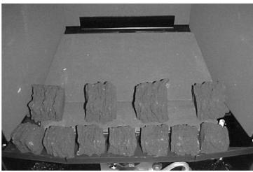
• Add 8 45mm x 45mm coals with rough faces upwards in lines behind the four placed in the last operation. It is VERY IMPORTANT for good flame picture and combustion that they are placed in rows with good spaces between. Make sure that the side rows are hard against the firebox sides. Place a further 3 45mm x 45mm coals behind these rows in the gaps as shown.
