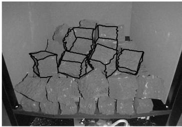
Add the 2 final 45mm x 45mm coals, 1 each side of the back pair of 55mm coals. Add the 2 final 35mm x 35mm coals on the back row as shown. The coal bed is now complete.
