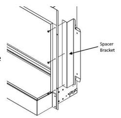
Fix the fire to the wall using 4 suitable screws and wall fixings. Use the holes in the spacer brackets as shown.
