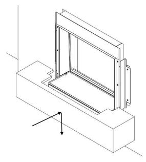
Now offer the surround up to the wall and lower into place to locate into the fixing brackets.
